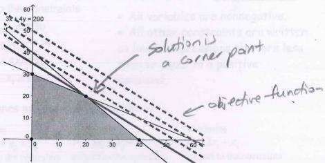
For higher dimensions with linear inequalities, the equations represent the equivalent of planes, and the feasible region is a multi-dimensions volume, but the solutions will still occur at corner points:
