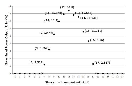
This graph shows power output from the solar panels vs. time in hours past midnight. Each point that is marked (t, P) gives the y-value (power, P) for a particular x-value (time, t).
