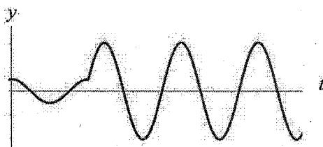
The mass initially oscillates at the natural frequency due to the initial displacement, and then when the mass is struck and new oscillation is started, also at the natural frequency by the impulse strike, beginning at the point where the mass was when struck.
