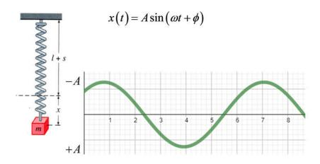
Because there are no other forces acting on the mass (there is no air resistance, and no energy lost to heat in the spring), this motion would (theoretically) occur unchanged forever.
