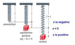
What we are usually interested in is the position of the mass over time, so we are using a differential equation with x as the dependent variable and t as the independent variable to find a solution function for x(t).
