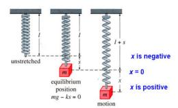
So now there are two forces acting on the mass: gravity and this additional force which stretches it further than equilibrium displacement to a distance of s + x.
