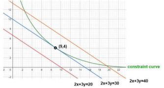
(iv) Objective function and constraint are parallel (tangent) at (9,4).
