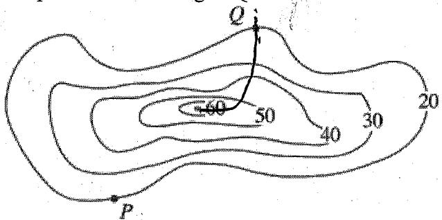
path must be perpendicular to contour lines
